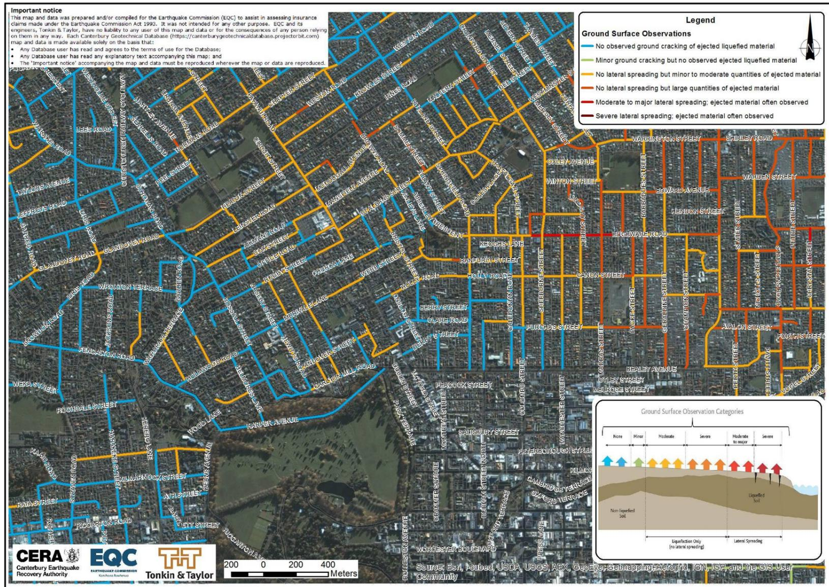
Figure 6 – Status of wastewater network as assessed at 20<sup>th</sup> April 2011 (NOW SUPERSEDED)
