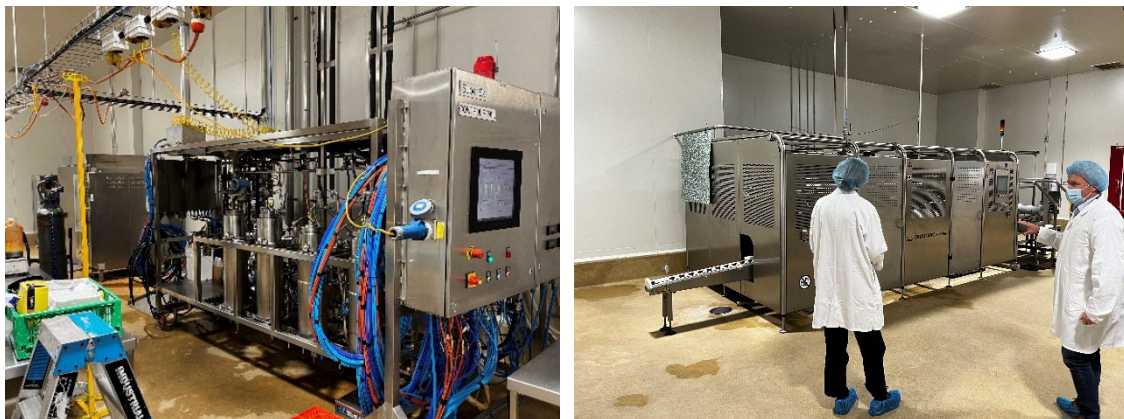
Figure 17 (left to right): CO 2 super critical extraction technology for extracting high value naturally occurring bioactives; FoodBowl Chief Executive, Grant Verry, shows the team a high pressure processing system, which can be used to non-thermally preserve food, extending shelf-life and preventing waste while maintaining the sensory and nutritional properties of the food product.
